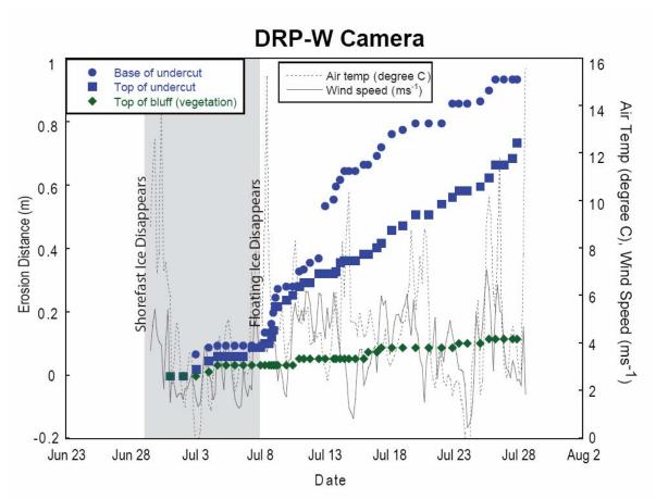
Figure 2 Rate of coastal erosion over July 2008 as reconstructed from time-lapse imagery at Drew Point. Erosion accelerates following retreat of sea ice, and is ongoing even in relatively calm wind conditions.
