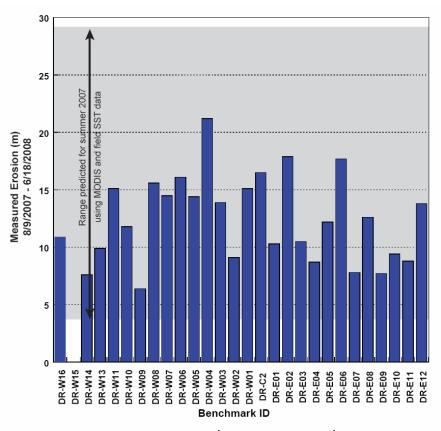
Figure 3 Integrated coastal loss over an entire season (9<sup>th</sup> of August 2007- 18<sup>th</sup> of June 2008) as reconstructed from repeat survey transect along Drew Point. Total loss is consistent with thermal erosion potential modeled from MODIS.
