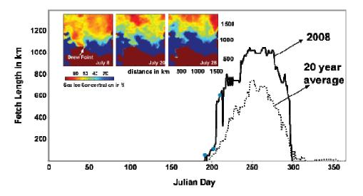
Figure 4 Fetch Length at Drew Point for different stages over the summer season 2008 is reconstructed from Nimbus-7 Passive microwave data, 2008 has open water distances that are 100's of km longer than the 20 year average conditions.
