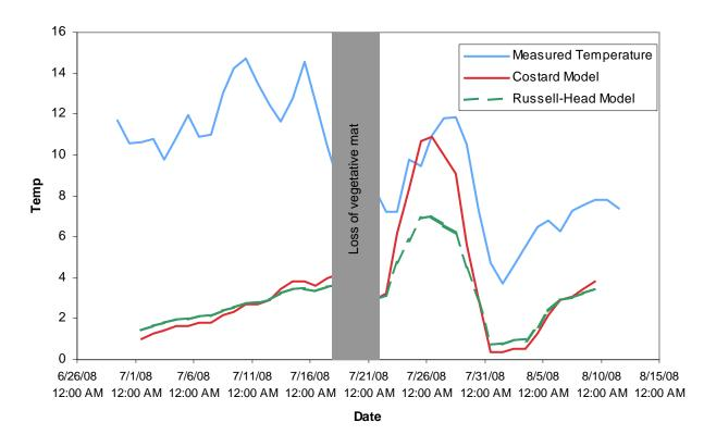
Figure 1 Modeled lake temperatures calculated from shoreline erosion rate mimic measured temperatures in the latter half of the summer of 2009.
