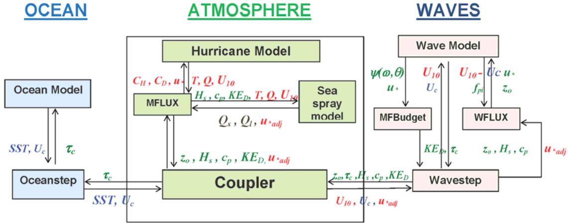
**Figure 1.** A schematic diagram of the coupled wind-wave-current modeling system and the air-sea interface module (ASIM) represented by the following components: MFLUX, Sea spray model, MFBudget, and WFLUX. The arrows indicate the prognostic variables that are passed between the model components.
