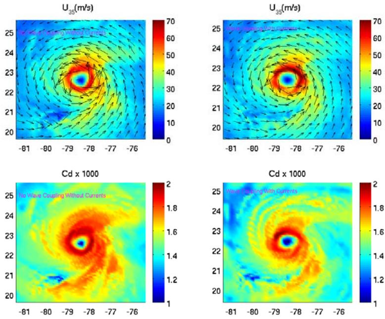
**Figure 5.** Wind speed at 35 m (the lowest model level) and drag coefficient in the control experiment (no wave coupling, no current effects) (top and bottom left) and with wave coupling and current effects (top and bottom right) at  $t=72$  hr.
