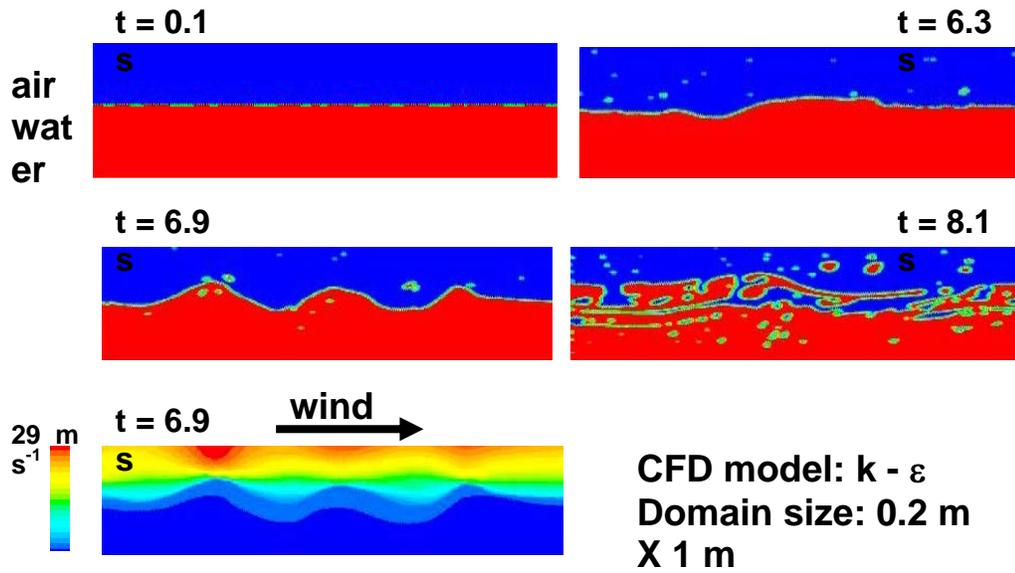
**Figure 8.** 2D simulation of the disruption of the air-sea interface and formation of a two-phase transition layer under hurricane force wind (Soloviev and Lukas 2010b).
