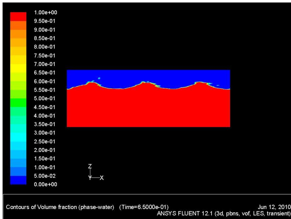
**Figure 9.** 3D simulation of the disruption of the air-sea interface and tearing of the wave crests due to the Kelvin-Helmholtz type instability at  $4 \text{ N/m}^2$  wind stress (side view).
