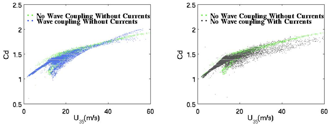
**Figure 4.** Drag coefficient vs. wind speed at 35 m in the coupled model experiments described in the text. Green dots are for no wave coupling/no current (control), blue dots are for wave coupling/without current, black dots are for no wave coupling/with current.
