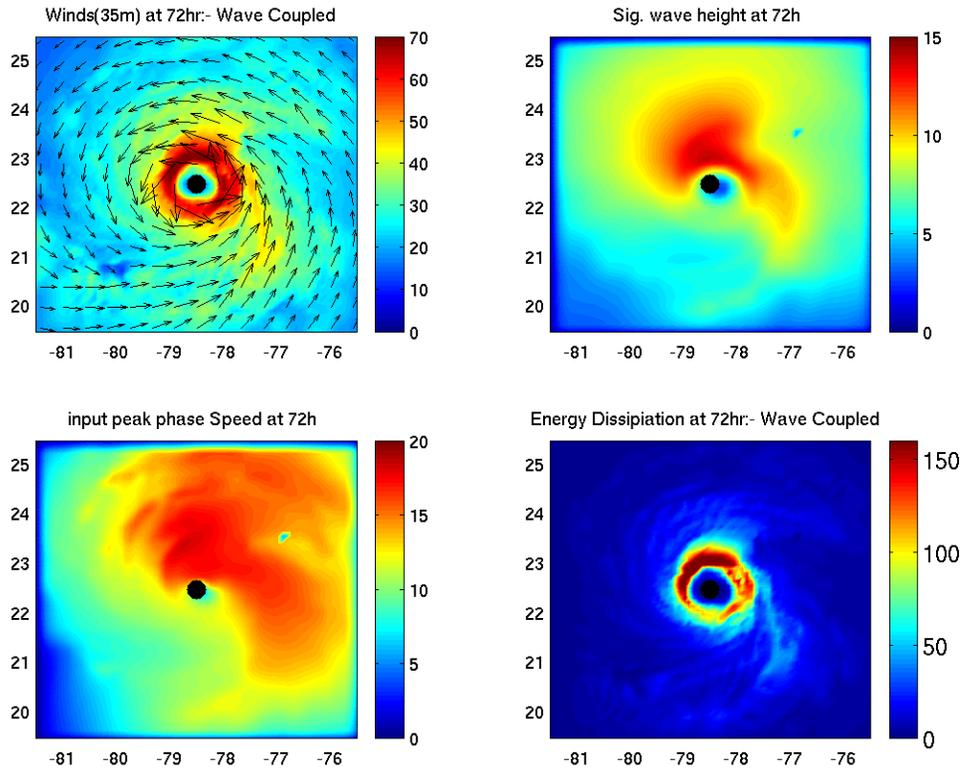
**Figure 2.** Surface wind, significant wave height, peak phase speed and energy dissipation due to wave breaking at  $t=72$  h in an idealized experiment using the GFDL coupled hurricane-wave-ocean system.
