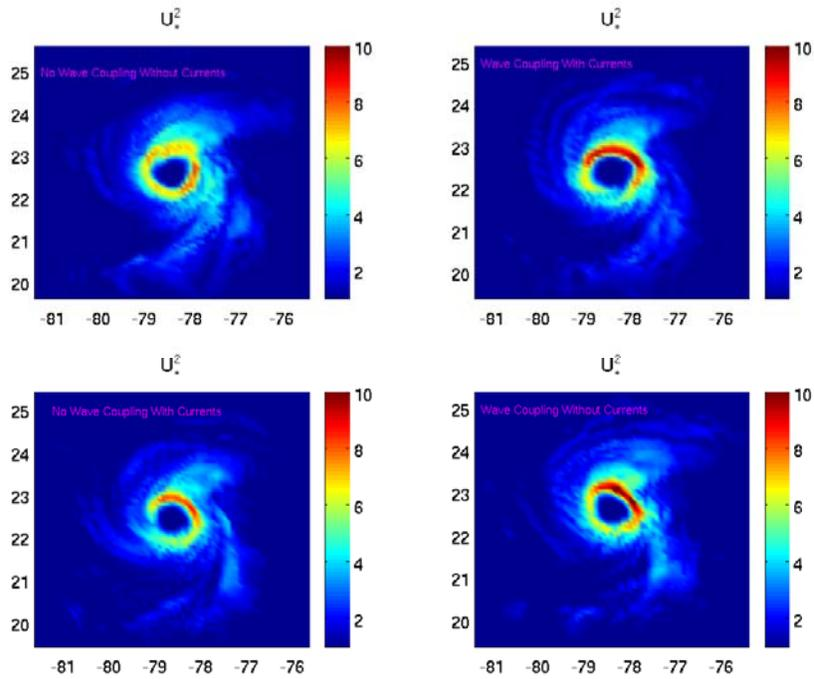
**Figure 6.** Normalized momentum flux ( $m^2/s^2$ ) in four sensitivity experiments: a) no wave coupling without current effects (top left), no wave coupling with current effect (bottom left), with wave coupling and with current effects (top right), and with wave coupling and without currents (bottom right) at  $t=72$  hr.
