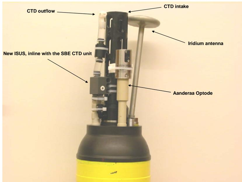
**FIGURE 2.** The upper endcap of a profiling float with the newly designed inline ISUS unit. This float was recently deployed at the HOT site near Hawaii.
