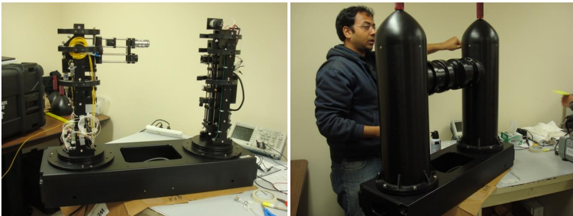
Figure 1. Internal electro-optical structure of the in-situ HOLOCAM (left panel). Pressure housings being assembled onto the first HOLOCAM (right panel).
