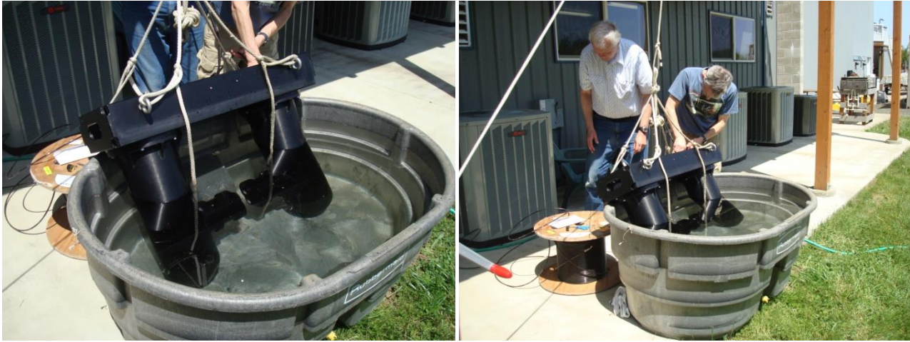
Figure 2. Submersion and system testing of the first HOLOCAM at WET Labs.
