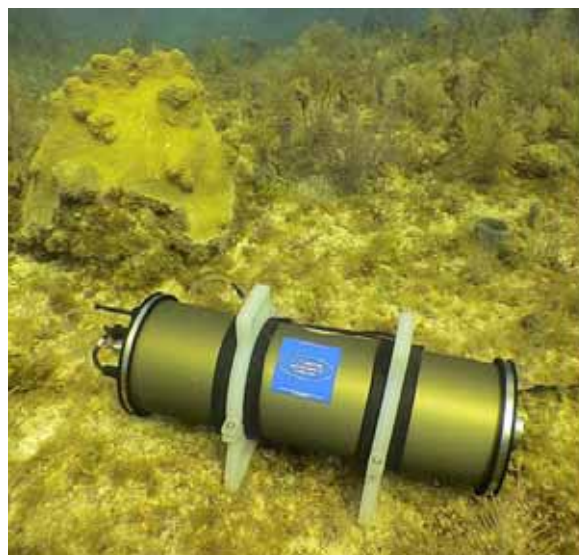
Figure 3: Above, photo of a TETHYS 100 meter unit during cabled observatory deployment at the Aquarius Habitat near Key Largo, Florida.
