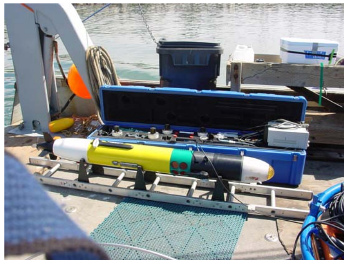
Figure 2. URI's REMUS vehicle with the MARCHEM ammonia analyzer payload ready for deployment from the R/V Shana Rae into Monterey Bay, CA.
