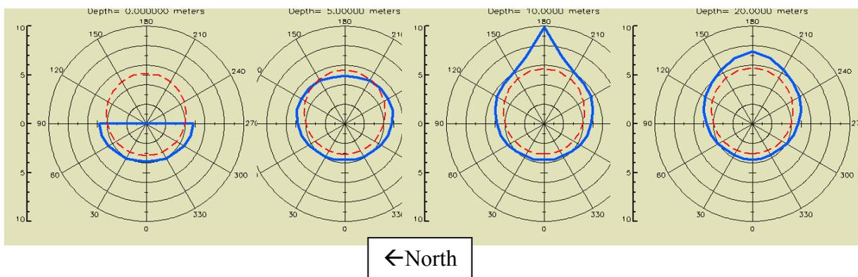
Figure 2. BIC results for simple case of homogeneous optical properties, sun angle directly overhead, and 0% reflective black target, at waters depths of 1, 5, 10, and 20 meters.
